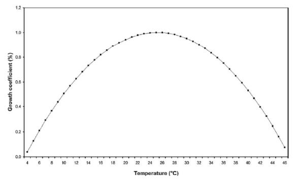
Fig. 1 – Leaf area function: hourly leaf area growth percentage in function of air temperature.
